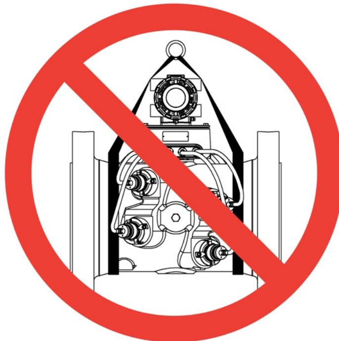
Figure 2-13 Incorrect sling attachment
