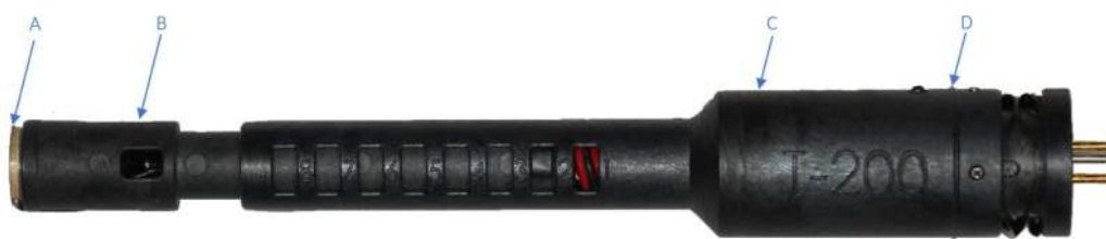
Figure 3-12: T-200 transducer capsule assembly identification
