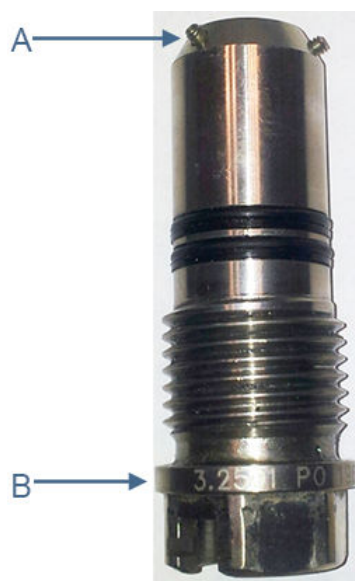
Figure 3-7: Transducer holder length and set screw identification
