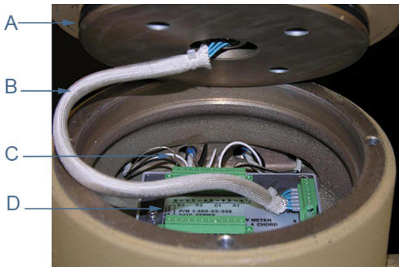
Figure 3-33: Acquisition Module cable and transducer wiring
