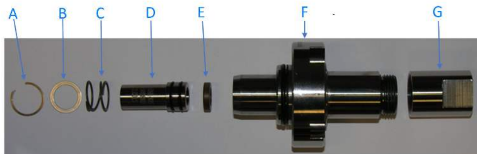
Figure 3-16: Components of the T-200 transducer assembly
