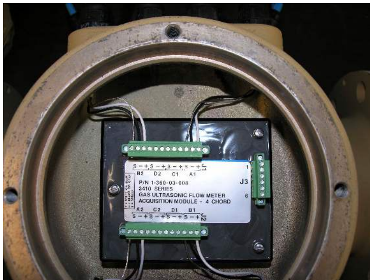
Figure 3-18: Model 3414 Ultrasonic Meter Acquisition Module wiring
