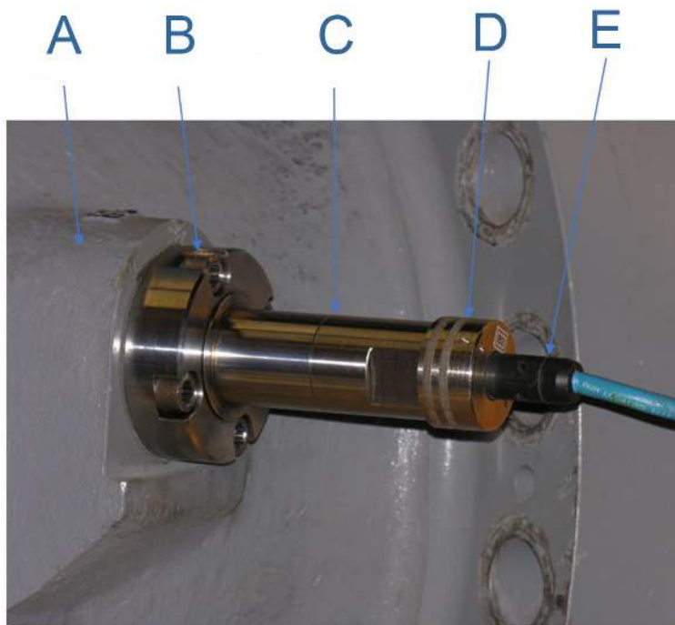
Figure 3-11: T-200 transducer assembly installed in a meter body
