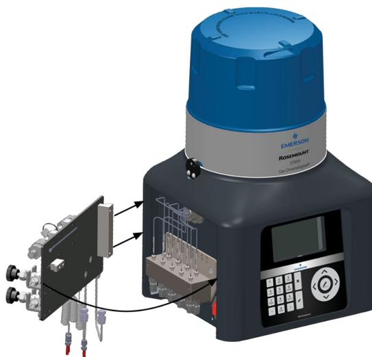
4. Slide the small mounting bar (1) to the right so that it fits behind the right edge of the cut-out. Tighten the small mounting block's screws.
