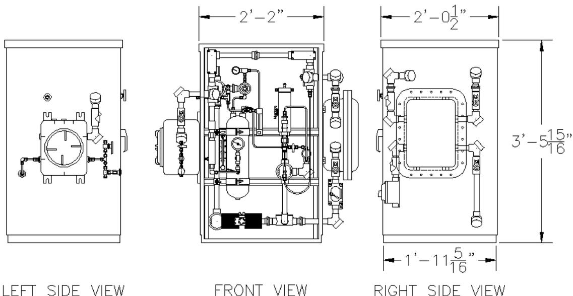
Fig. 1a—Mustang Intelligent Vaporizer Sampling System® Model 2
