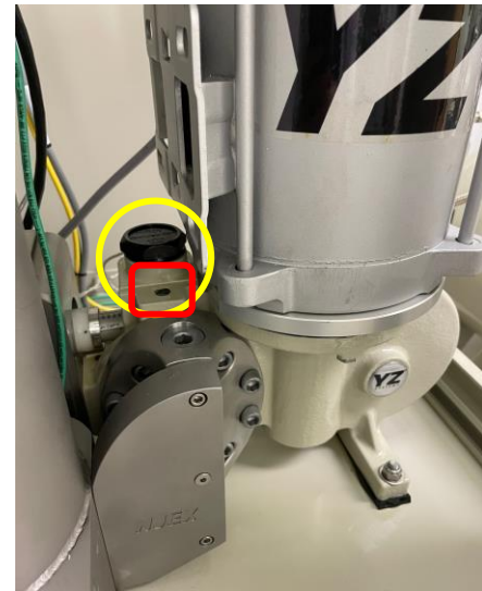
Figure 52 Oil Reservoir Cap Location (Yellow) and Pressure Relief (Red)
