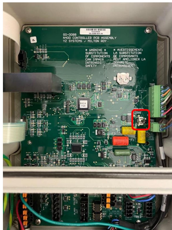
Figure 16 Controller board component layout with power switch location highlighted in a red rectangle.
