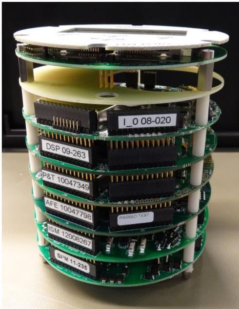
Figure 4: FGM 160 flow computer electronic modules.
